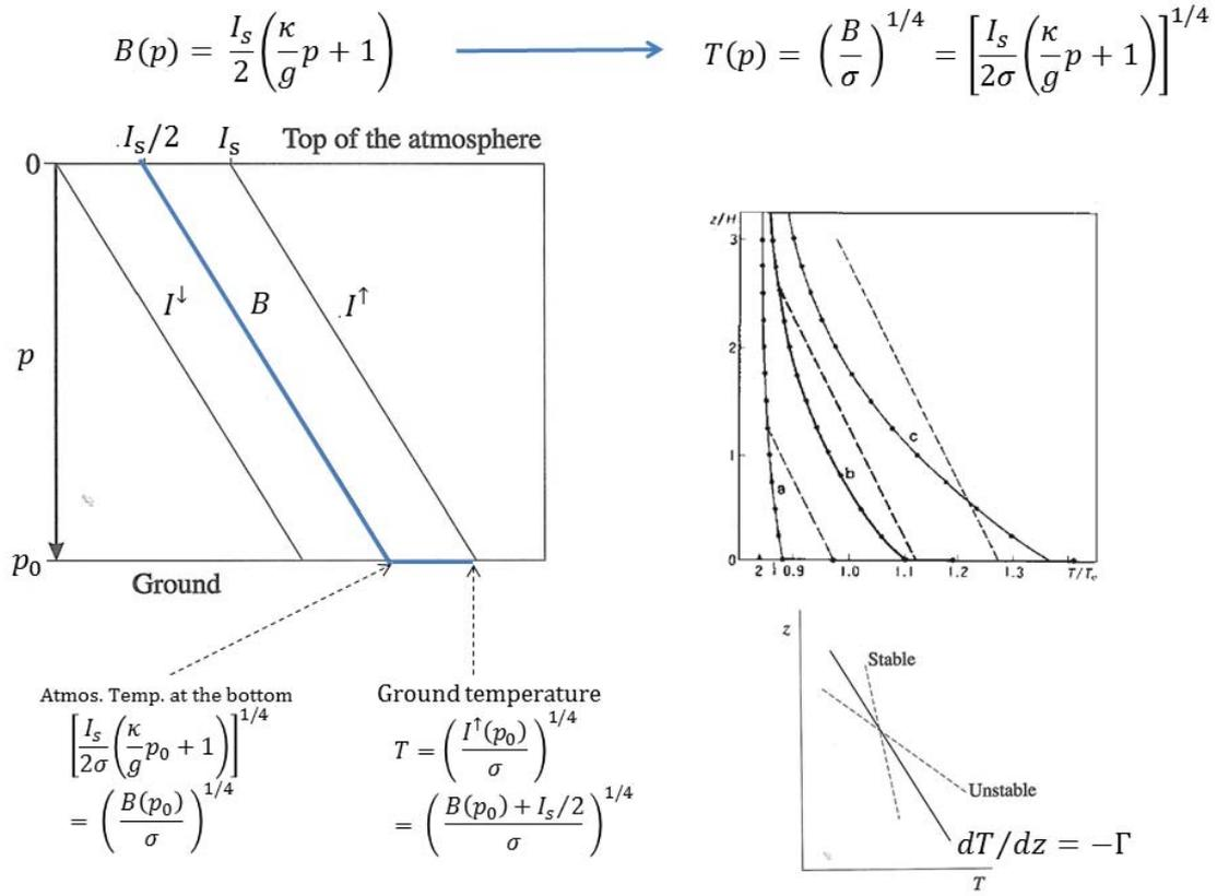
**Fig. 3.2** Radiative equilibrium temperature profile in  $p$ - $T^4$  space with a gap at the ground (left) and in  $z$ - $T$  space with convectively neutral adjustment in a layer above the ground (right),
