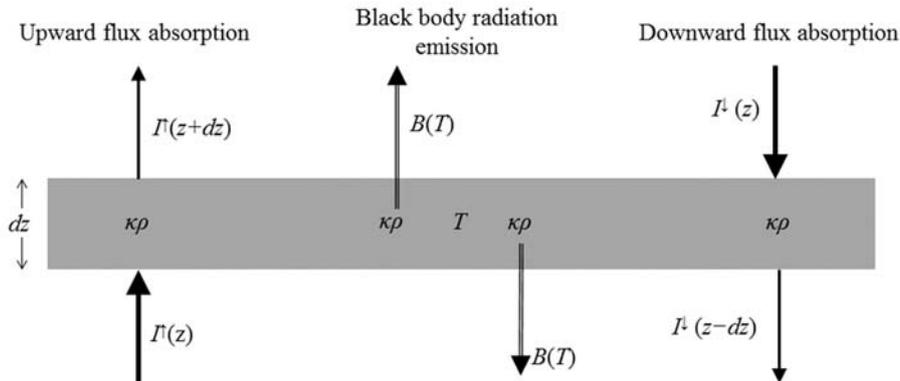
**Fig. 3.1** Two stream approximation in a gray body atmosphere.
