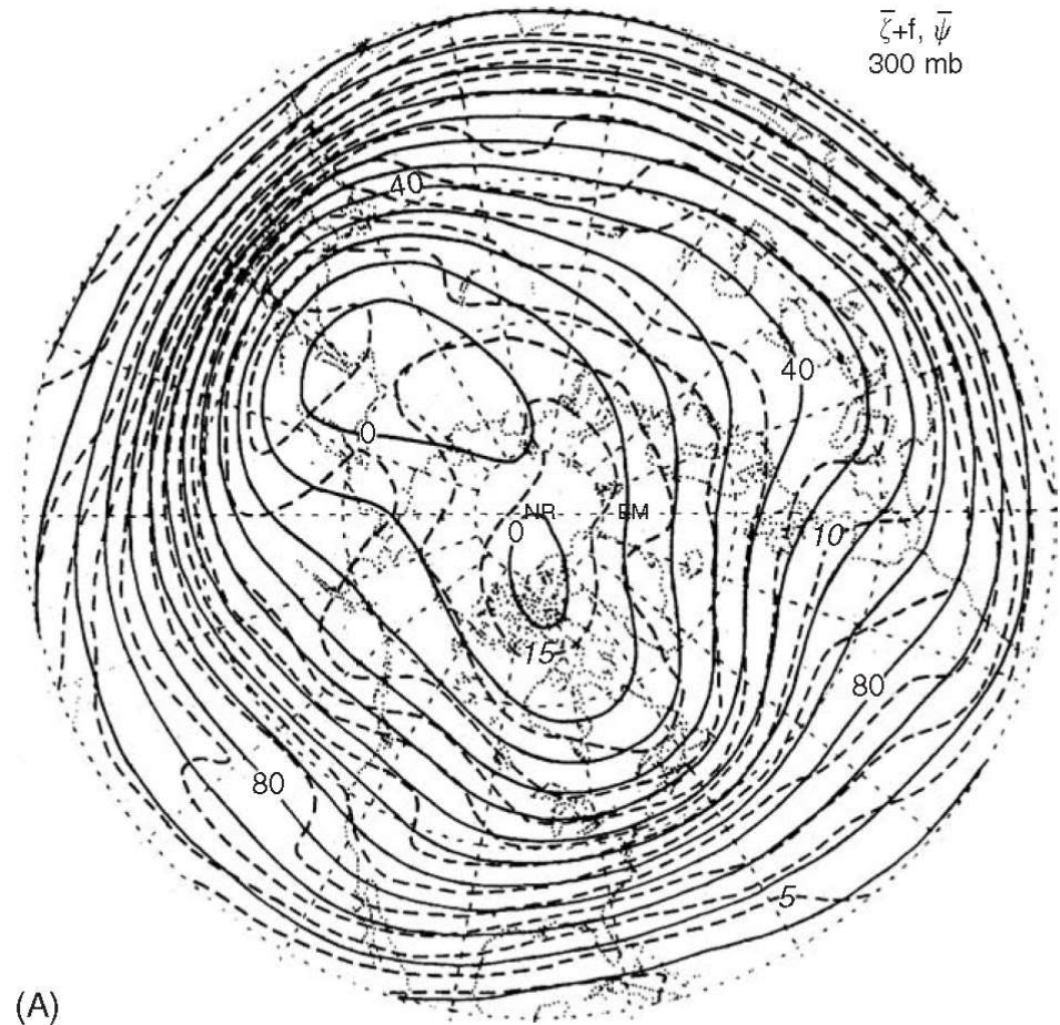
Figure 2 (A) Streamlines (solid) and absolute vorticity, \zeta + f , averaged at the 300 hPa level in the upper troposphere (figure from Lau NC, Journal of the Atmospheric Sciences , 36: 996–1016, 1979). The deviation of the streamlines from circles is a wave pattern analogous to Figure 1 . If this were simply barotropic Rossby waves, the dashed and full lines would coincide. Continents are shown with dotted curves; North America is at the bottom of the figure.
